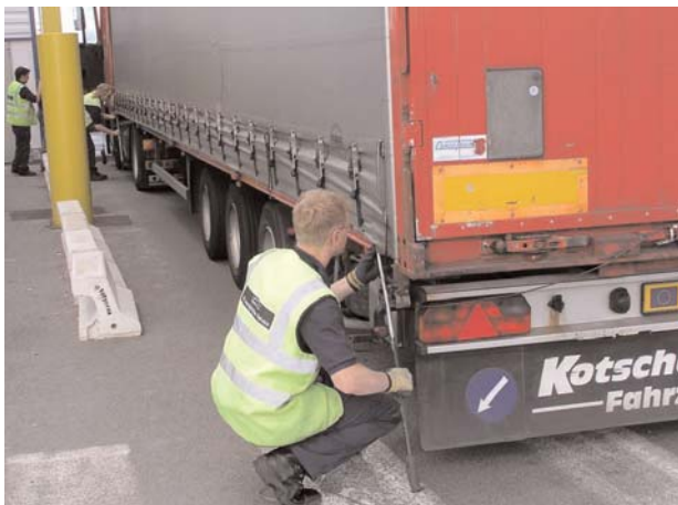
Immigration officers check a lorry for stowaways at a port, using carbon dioxide detection equipment
